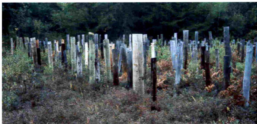
Forintek's fence post tests in Petawawa, Ontario.
